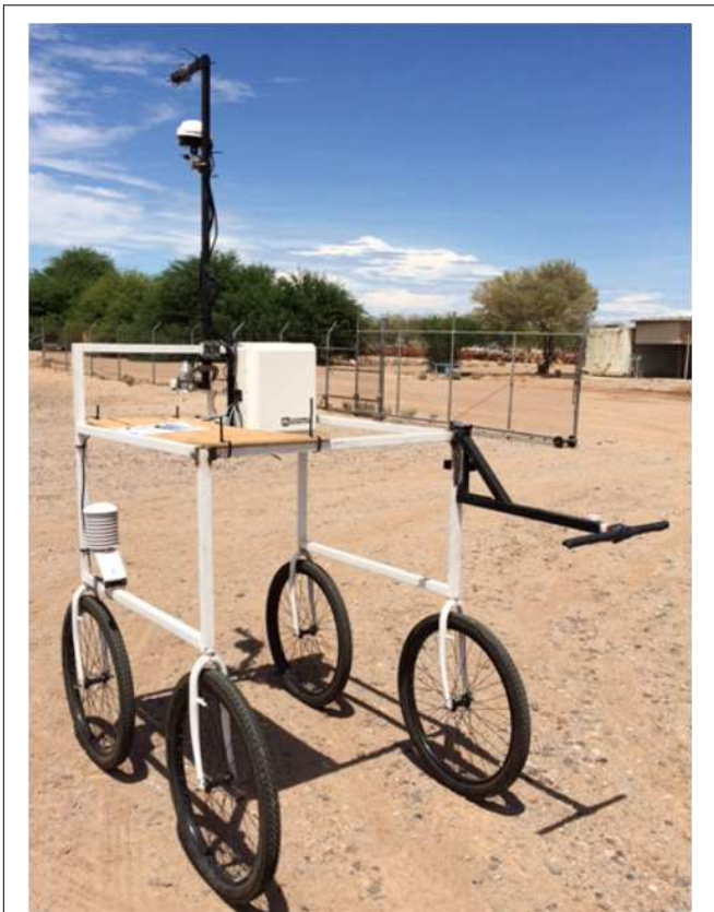
FIGURE 1 | Proximal sensing cart with a sensor bar, data logger, sensors, and extended handle. Camera sensor bar and cameras are not shown.
